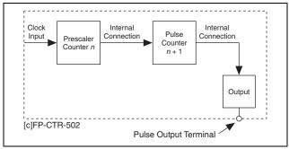
Figure 11. Continuous Pulse Train
